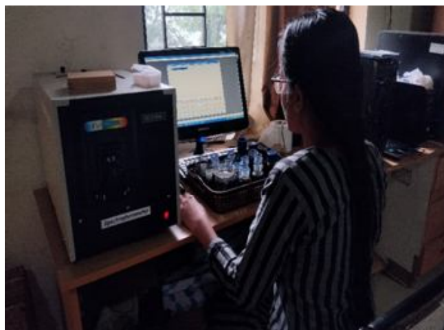
Plate 2 : Colour strength and colourcoordinates assessment of extracted dye liquids
